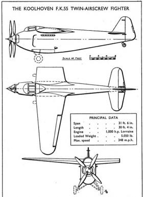
A General Arrangement Drawing of the Koolhoven F.K.55 Fighter, drawn to a 1/72nd scale. If a larger-sized model is required, scaling-up may easily be effected with the aid of the scale-rule shown above
